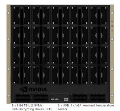
Power button / Status LED Unit Identification (UID) button / LED Fault LED indicator
