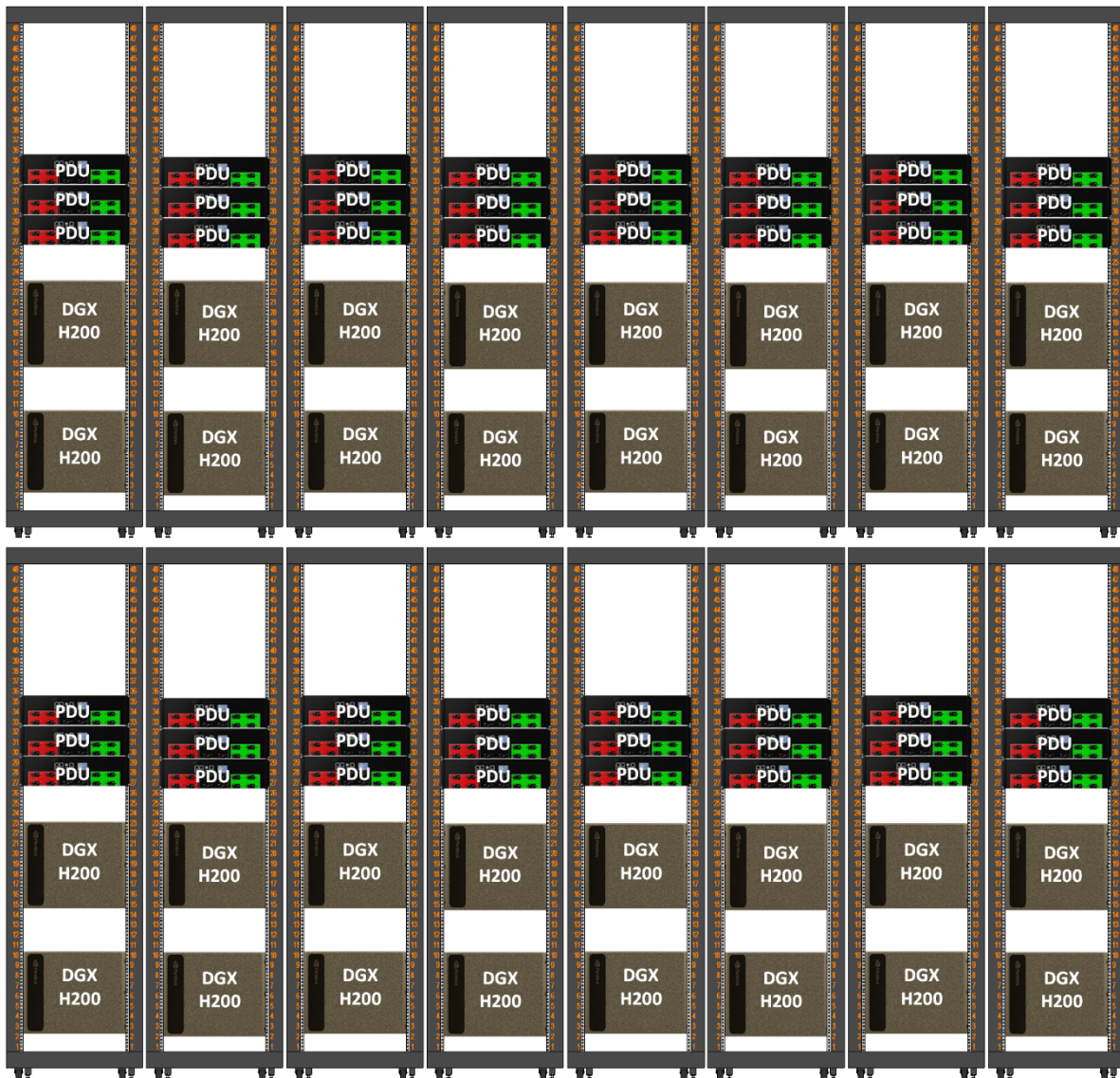
Figure 2. Complete single SU rack layout
