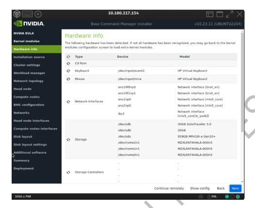
For example, that the target storage device and the cabled host network interfaces are present (in this case three NVMe drives are the target storage device, and ens1np0 and ens2np01 are the cabled host network interfaces).
